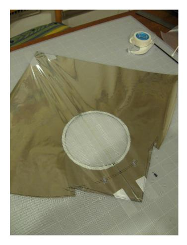
18.. Starting at the nose end, lay the spine onto the centerline exactly between the guide marks you drew earlier. Once the spine is down, remove tape from the sail, flip it over, and use your finger to burnish the sail onto the spine.
