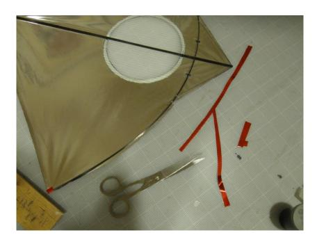
32. Carefully wrap the flap over the bow, making it as smooth as possible. Using your fingers, make sure that the sail is well adhered to the bow. Clean off any excess contact cement on the sail.
